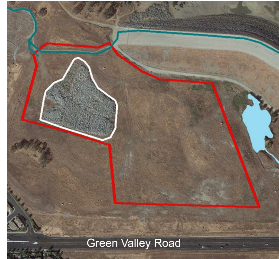
Work limits for the rock processing indicated in red.
